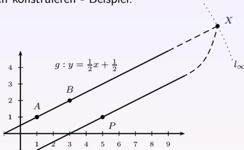
$$\Rightarrow \text{parallel}(g, P) := \text{join}(\text{meet}(g, l_\infty), P)$$
